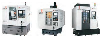
1. GLASS-600 Class CNC Machining Center are especially for the material such as ceramic, panel glass in 3C industry like mobile phone panel glass, PC panel glass and GPS navigator touch panel, etc. Besides, this machine can provide the solution for the electric resistance plate shaping. It has multi functions, mainly on polishing, slotting, drilling and chamfering and trimming and etc.
