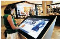
Zytronic's patented MPCT™ touch technology is capable of detecting 40 or more touch events at once. And there's no compromise on accuracy, even at ultra large sizes up to 85". MPCT™ multi-touch sensors are capable of millisecond-fast response speeds and excellent touch-point resolution.
