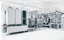
SmartWeb® is the benchmark roll-to-roll sputter system for touch panel, optical multilayers and barrier coatings.
